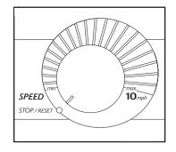
**before the walking belt can be restarted.** Next, slowly turn the speed control until the walking belt begins to move at slow speed. Carefully step onto the walking belt and begin exercising. Change the speed of the walking belt as desired by turning the speed control.
